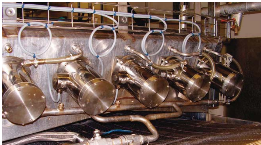
Marlin motors before and after steam cleaning on the Twiglet line.
